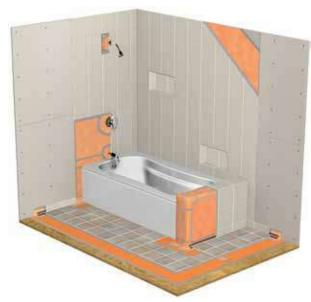
Waterproofing is the foundation of successful tiled bathrooms. Moisturesensitive construction materials (e.g., wood framing, plywood and OSB sheathing, gypsum wallboard, etc.) are common in the North American building environment and must be protected in wet areas. Wet areas also bring the potential for mold growth if effective moisture management is not provided. The key to mold control is moisture control.
