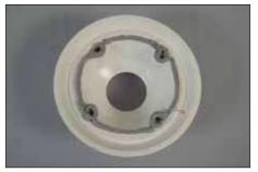
Apply a 1/4" - 3/8" (6 mm - 10 mm) bead of KERDI-FIX to the installed drain flange. Place the adaptor ring on the installed drain, re-insert the bolts, and tighten evenly. Make bolts finger-tight plus 1/4 turn; over tightening may warp the ring and result in leaks.
