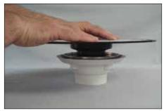
Slide the adaptor flange into the adaptor ring and ensure full support underneath with mortar or the detachable center section of the foam tray. Depending on the installed drain elevation, it may be necessary to install a polystyrene foam panel, tile backerboard, etc. prior to the tray. Install the tray as per the instructions on page 22.
