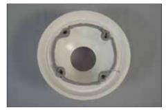
2 Apply a 1/4" - 3/8" (6 mm - 10 mm) bead of KERDI-FIX to the installed drain flange. Place the adaptor ring on the installed drain, re-insert the bolts, and tighten evenly. Make bolts finger-tight plus 1/4 turn; over tightening may warp the ring and result in leaks.
