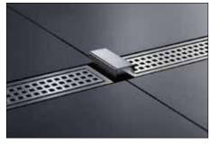
Apply a sufficient amount of thin-set mortar to the substrate and/or the back of KERDI-LINE-FC and press the profile into the mortar until its surface is flush with the adjacent tile and grate assembly. Leave a space of approximately 1/16" – 1/8" (1.5 – 3 mm). Fill the joints completely with grout or setting material.
