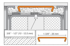
Install KERDI-LINE channel bodies end-to-end and overlap the KERDI collars using Schluter SET™, ALL-SET™, FAST-SET™, or unmodified thin-set mortar to ensure a waterproof connection.
